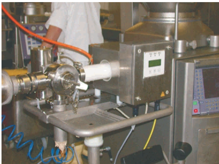
Metal Separator P-TRON 02 O 65 installed on a Vacuum Filler
